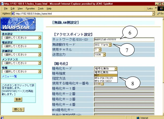
6. Confirm the ESS-ID\* (Network ID) of your wireless LAN network at the [ネットワーク名(ESS-ID)] (ex. "WARPSTAR-FFFFFF").
